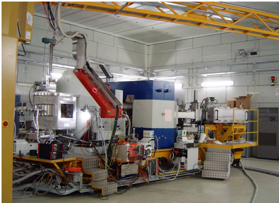
Figure 4.2: The MAGNEX spectrometer installed at LNS-INFN. The two large magnets, the dipole (white-red) and the quadrupole (blue-white) are visible. The focal plane detector is located after the quadrupole, on the right side of the picture.
