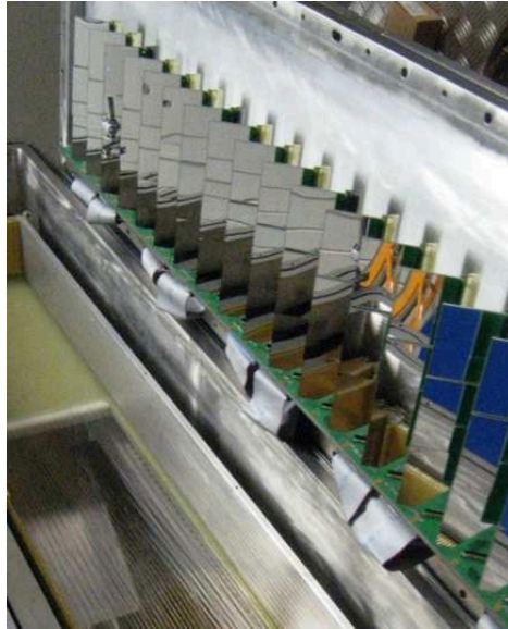
Figure 4.6: The MAGNEX FPD silicon detectors. The columns are rotated in order to let the detectors show their active area perpendicular to the reference trajectory.
