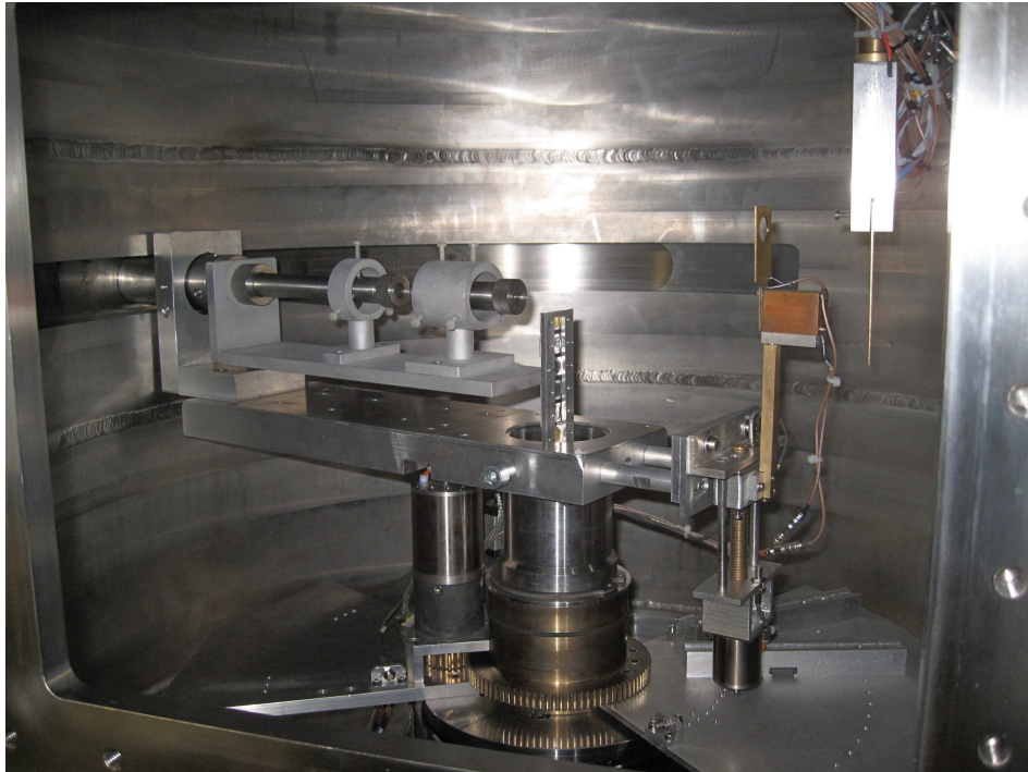
Figure 4.1: A picture of the scattering chamber. The collimation system, the target ladder and the Faraday cup are visible.
