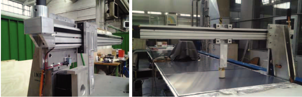
Figure 5.4: Mechanical arm that carries the source during the scan.
