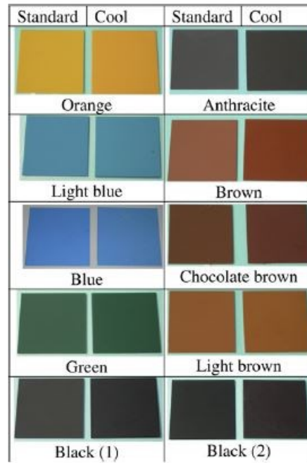
FIGURE 3.7: Standard and cool coatings for pavement tiles tested at the University of Athens [17]
