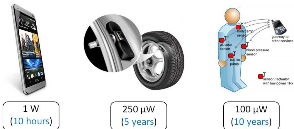
Fig. 1.3. Power requirements and lifetime of typical WSN products.
