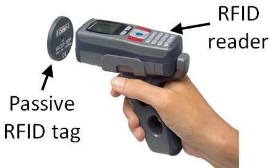
Fig. 1.4. Passive RFID tag and reader.
