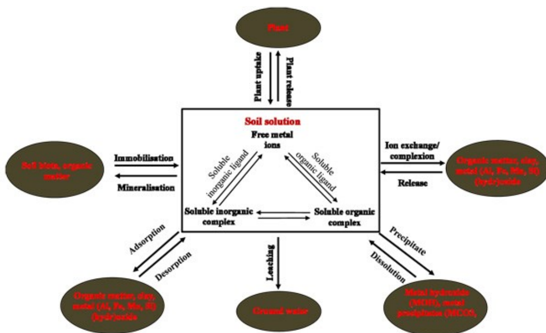
Figure 7. Various chemical and physical pathways a metal ion may encounter once introduced into the soil environment.
