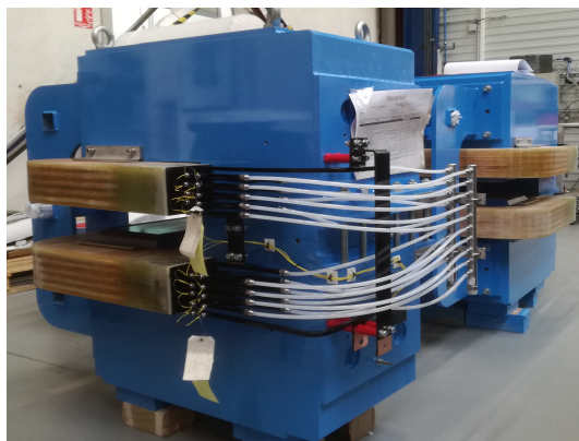
Figure 2.12: Picture of the dipoles during the assembly at SigmaPhi company.
