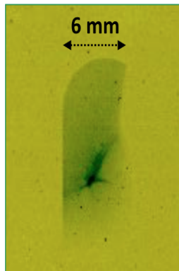
Figure 5.31: RCF-EBT3 irradiated in position P1 after PMQs set to focus 7 MeV protons at 44 cm from the target.
