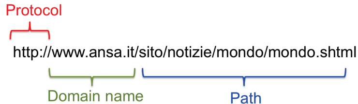
Figure 2.1: Components of a URL: protocol, domain name and path of a Web resource.
