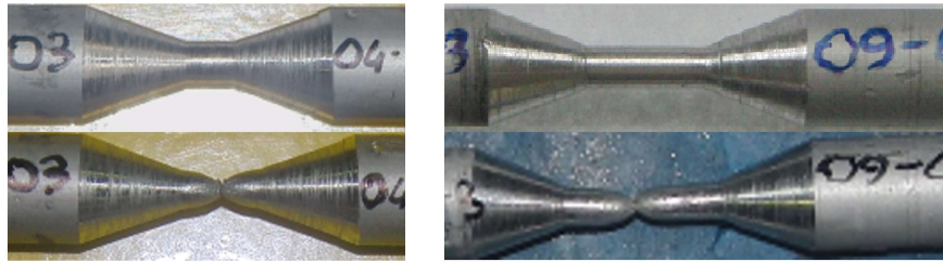
Figure 3.7: Neck-affected zone in short and long specimens
