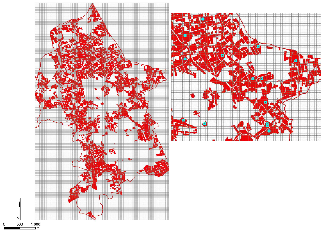
Fig. 5.2 - The overlaid sampling grid on semi-detached house land use (left) and a detail of the random generated sampling cells (right) for the municipality of Mascalucia
