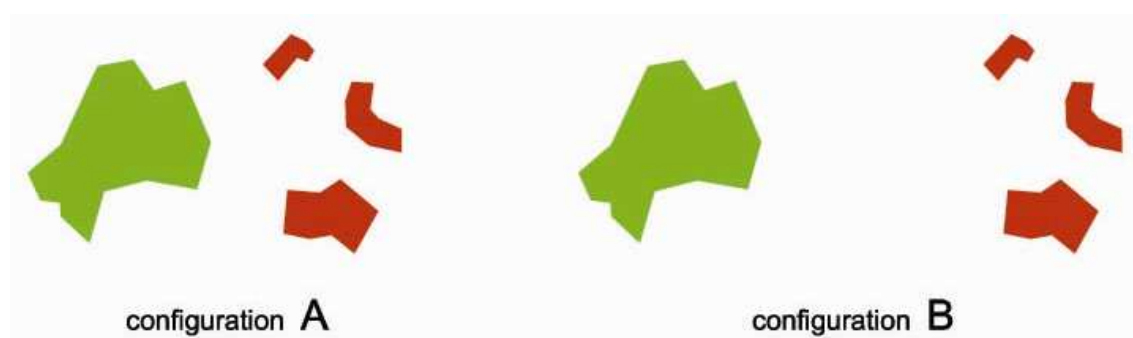
Fig. 5.11 - Example of proximity modelling: in the configuration A the NUA in green has a higher proximity to the 3 residential areas in red than in configuration B.
