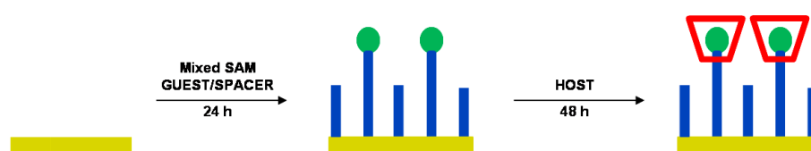
Figure 58. Schematic rappresentation of directly complexation on surface.
