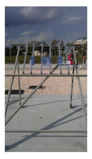
Figure 5. 87 External bench for outdoor exposure test
