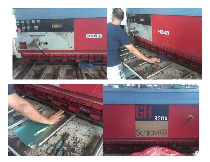
Picture 5. 1 Some shots while cutting the aluminum mirrors and the PF mirror
