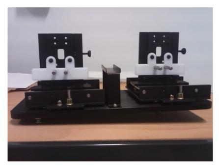
Figure 4. 4 Spectrophotometer sample holder, one for the reference beam and the other for the sample beam
