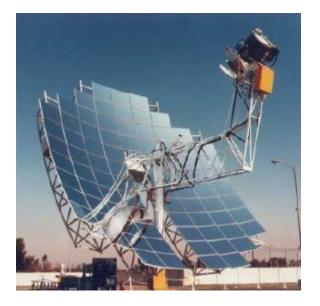
Figure 2. 3 SES Dish/Stirling system
