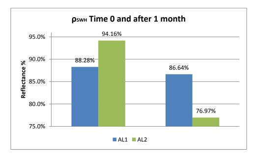
Figure 5. 132 Comparison between the solar weighted hemispherical reflectance for AL1 and AL2 sample in the "before" and "after" condition
