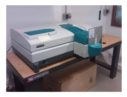
Figure 4. 1 Spectrophotometer Agilent Cary 5000
