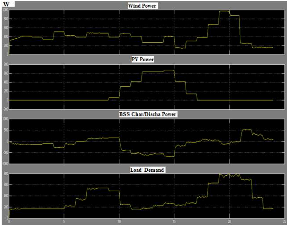
Figure 3.3. Simulation results of PVG/WEG/BSS hybrid generator
