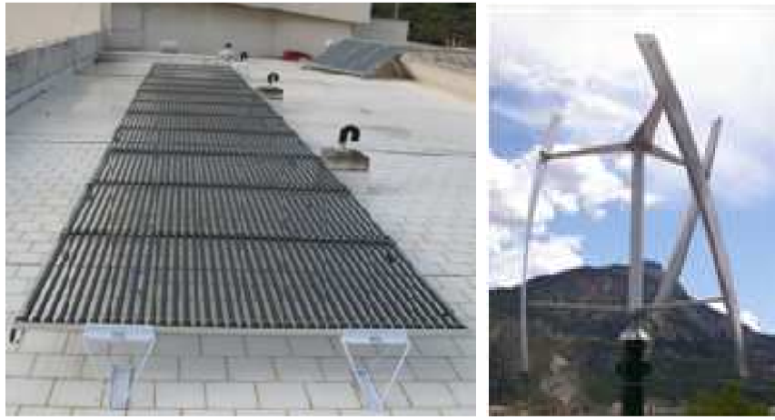
Figure 3.14 Solyndra PV arrays and TN-1.5 Tozzi Nord mini wind turbine installed in the lab
